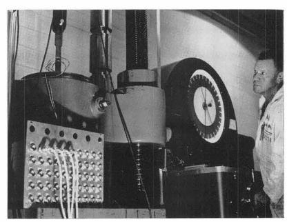
STEEL TENSILE SPECIMEN, center left, is set up for a "pulltest" which can be as great as 300,000 lbs. Operator is Andy Imrisek.
